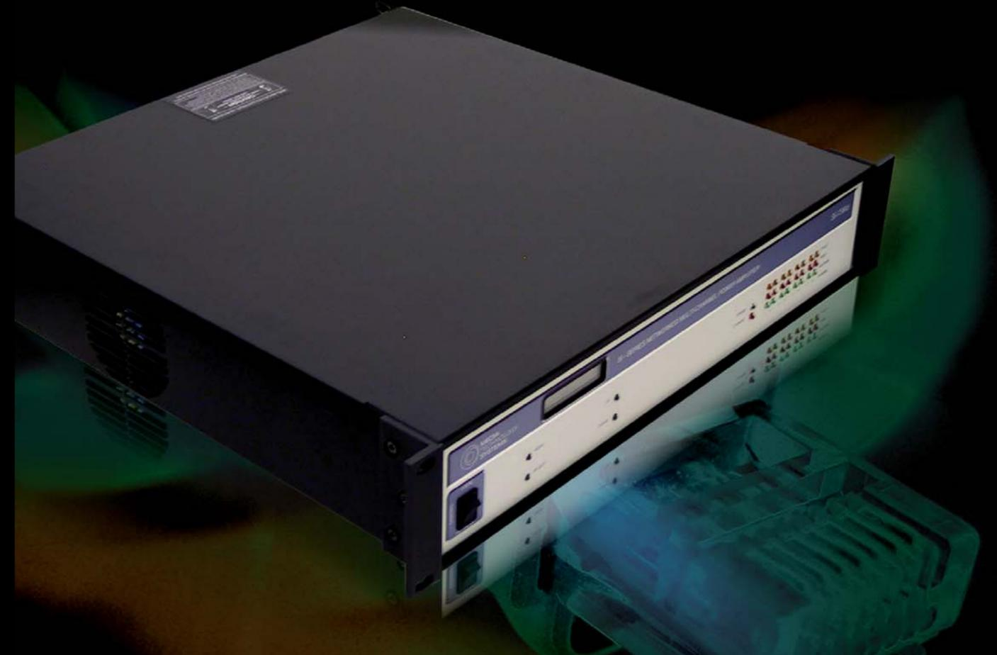
The SI-series amplifiers employ a Class D output topology for maximum efficiency and does not require high volume, forced fan cooling even with the amplifier running into clip on all channels. In addition, the switch mode power supply (SMPS) incorporates power factor correction (PFC) to comply with incoming legislation and minimize noise pollution of the electrical supply.
