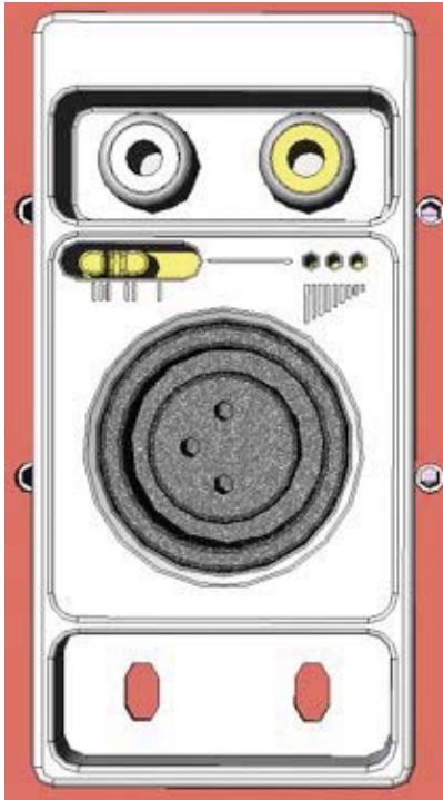
Figure 3-4: Graphic showing ION2.0 label recess (bottom of fascia plate) with label screw holes.
