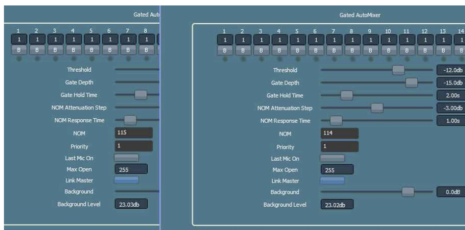
Figure 6-16: Automixer linking fault – both devices set to Master
