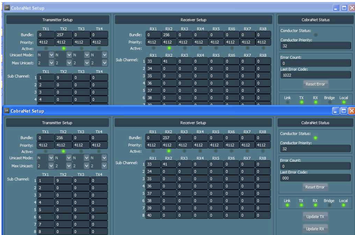
Figure 6-5: Screenshot showing how to link control signals between two AMX8.8CN
